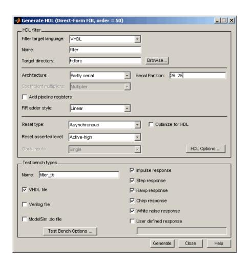
**Note** The **Architecture** pop-up menu also includes the new Distributed arithmetic (DA) option (see "Distributed Arithmetic Support for FIR Filters" on page 19).
