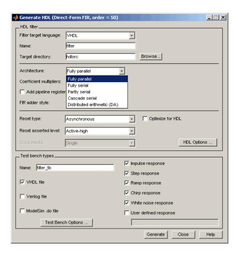
When the Partly serial or Cascade serial option is selected, the Generate HDL dialog box displays the **Serial Partition** field (shown in the following figure). See "Speed vs. Area Optimizations for FIR Filters" in the Filter Design HDL Coder User's Guide for a full description of serial and parallel architecture options.
