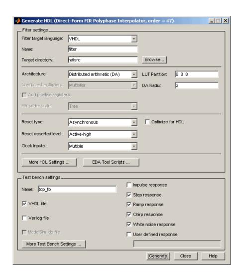
**Note** For multirate filters with the Partly serial architecture option selected, the **Clock inputs** options is set to Single and disabled.
